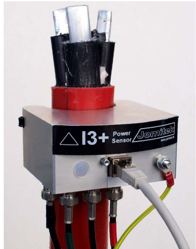
Illustration 5: A combined current and voltage sensor. The capacitive voltage input is via the BNC connectors in the bottom.
