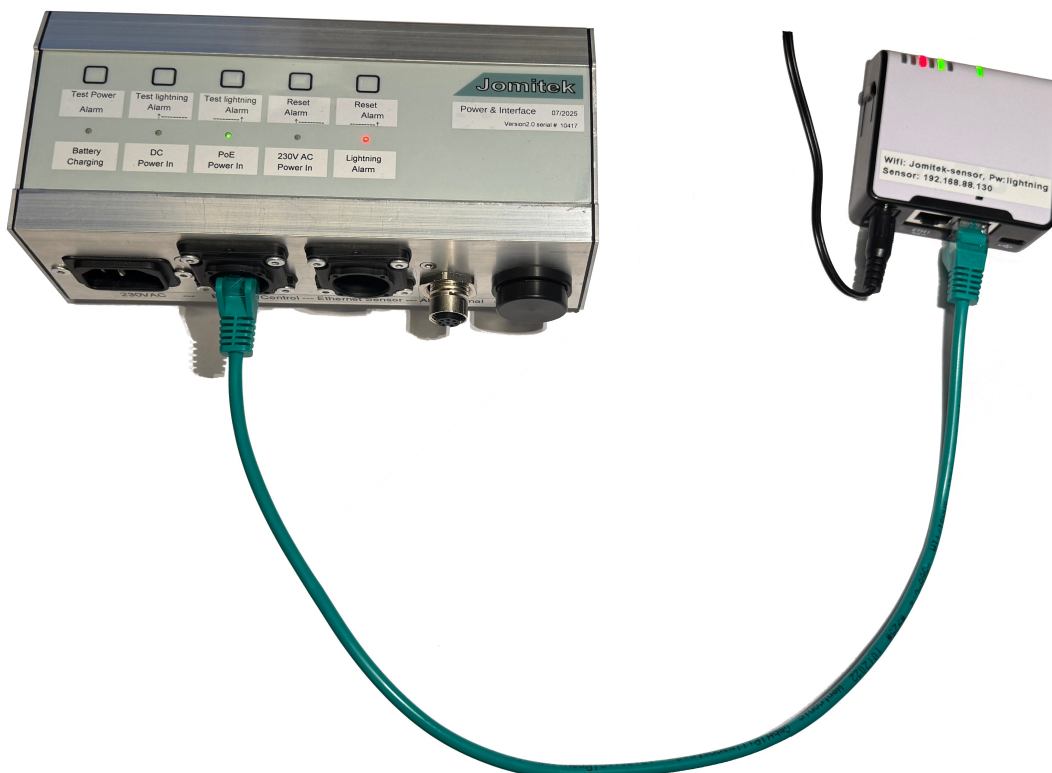
The EPS (right hand side), connected to and powering a Power and Interface Box. Connection from PIB to LSA not shown.
