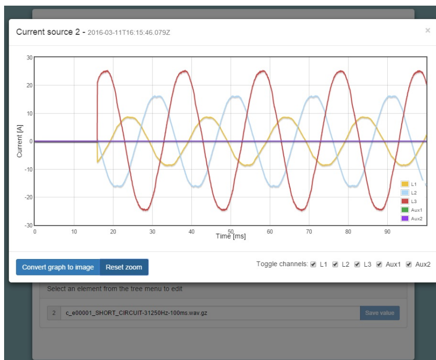
Figure 32: View of one of the data files of a short circuit event, tested with a short circuit threshold of 5Ampere.
