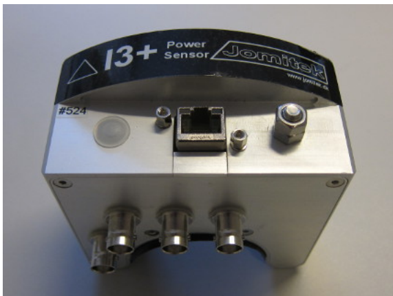
Figure 2: Front and bottom view of the I3 sensor showing the PoE connector, grounding bolt and voltage measurement BNC connectors.
