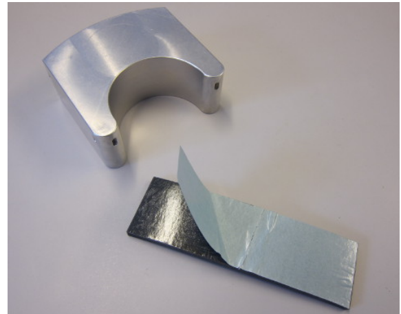
Figure 13: Use the adhesive rubber patch to line the sensor.
