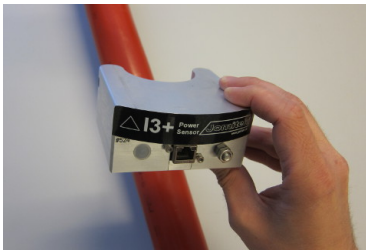
Figure 6: Place the sensor on the cable to be measured.
