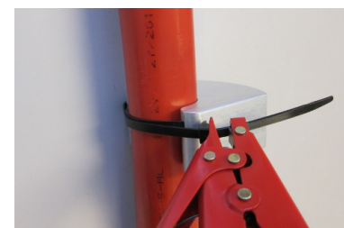
Figure 11: Use the provided tool to tighten the cable tie.
