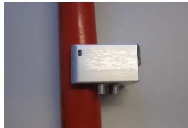
Figure 7: Make sure that the sensor is mounted such that the voltage BNC connectors are facing down.
