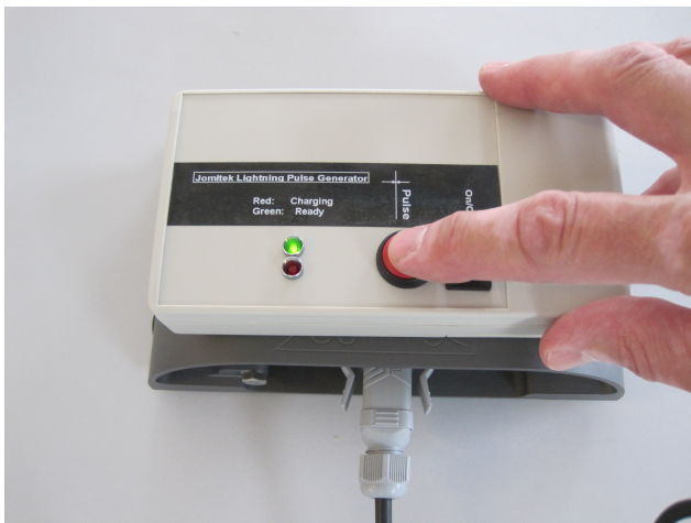
Lightning test generator placed on top of the sensor.
