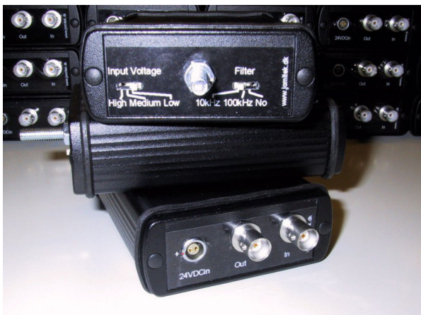
Figure 10, Measuring amplifiers for measurement at very high frequencies
