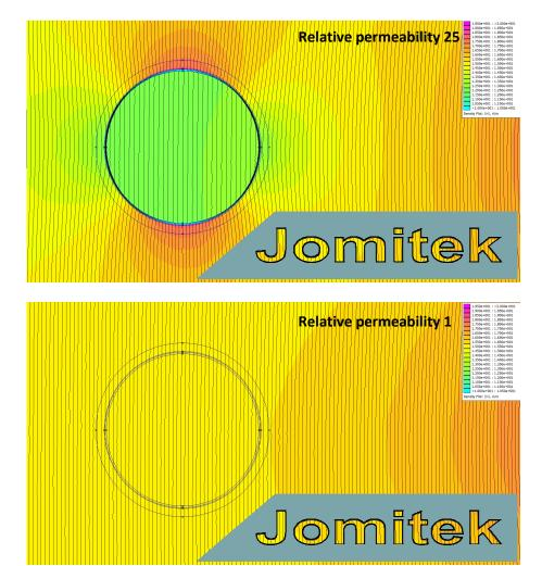
The lightning sensor measures the magnetic field created by the lightning current tangentially and horizontally to the surface of a wind turbine tower at a distance of 3cm. The following graph presents the magnitude of the tangential field relative to the maximum tangential magnitude in the simulation with permeability 1:
