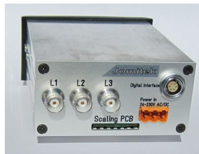
The 3 inputs are connected to the 3 capacitive connections on the bushings
