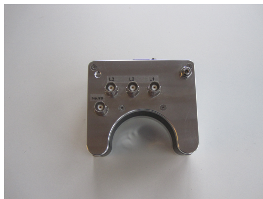
Figure 3: Voltage measurement BNC connectors. The default channel usage starting from the lower left going up to the right is: neutral, L3, L2, L1.
