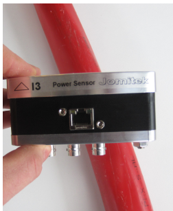
Figure 6: Place the sensor on the cable to be measured.
