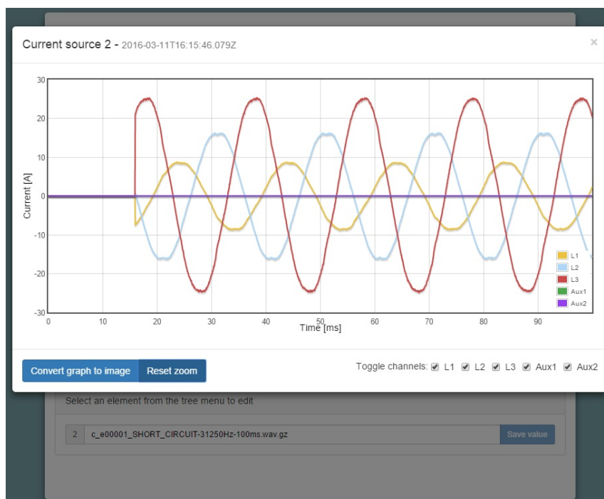
Figure 25: View of one of the data files of an over current event, tested with a threshold of 5 A.
