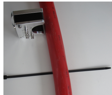
Figure 8: Wrap the cable tie around the cable to be measured.
