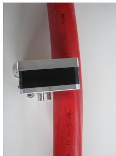
Figure 7: Make sure that the sensor is mounted such that the voltage BNC connectors are facing down.
