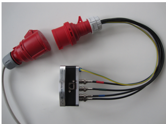
Figure 4: Capacitive voltage measurement interface attached to the Jomitek I3 Power Sensor . The CEE adapter is shown to the left.
