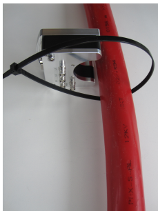
Figure 9: Wrap the cable tie around the cable and thread it through the cutout on the opposite side of the sensor.
