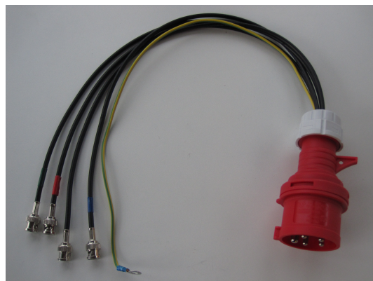
Figure 5: CEE connector for use with the capacitive voltage measurement interface. Note the integrated ground connector.
