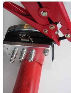
Figure 11: Use the provided tool to tighten the cable tie.
