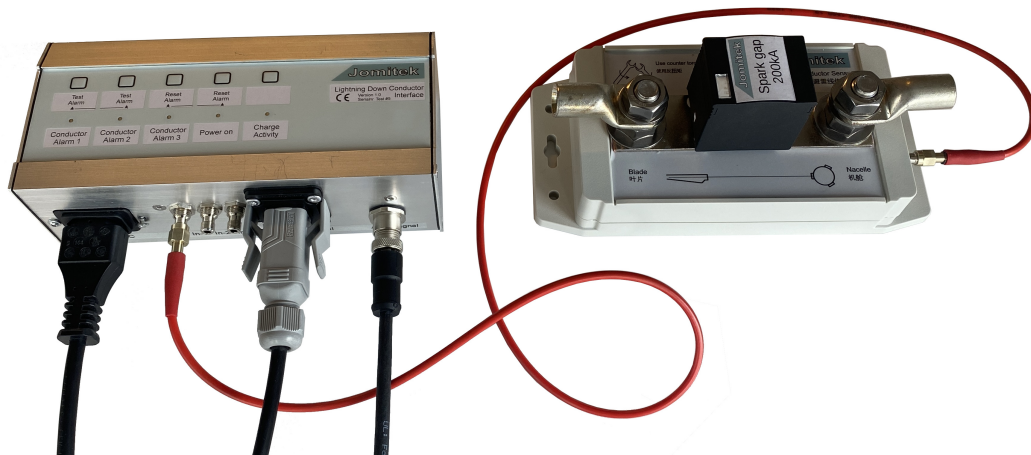
Figure 3: Full system, with one sensor connected, including frontpanel buttons and LED indicators.
