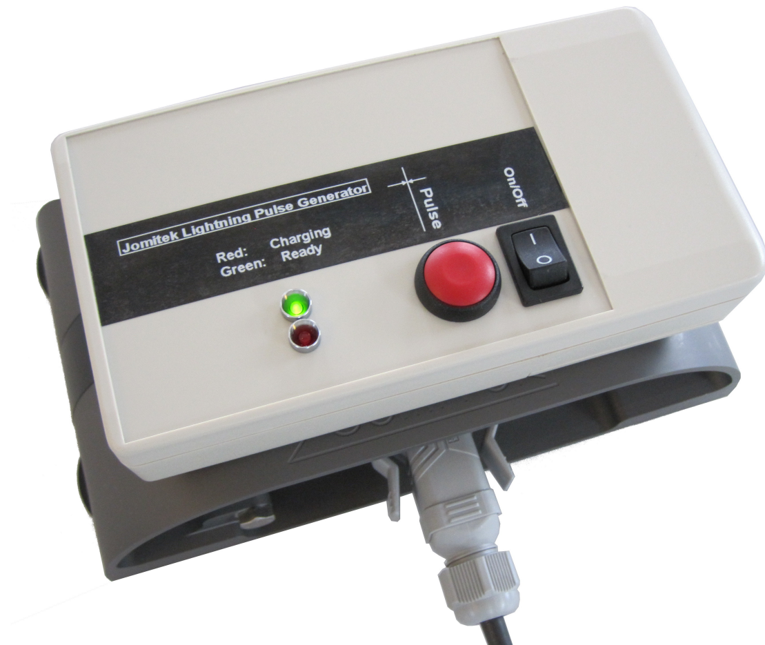
Figure 9: The Jomitek Lightning Pulse Generator must be placed centered and on top of the LSA box, to allow for correct detection of the test pulse.
