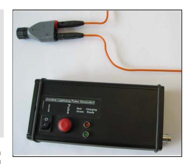
By holding this loop close to the individual antenna under test, the generated field will be applied to the sensor antenna.
