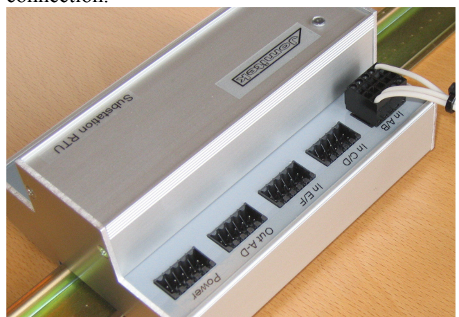
Figure 3, RTU using cage clamps, Here it is from the vendor Weidmüller.
